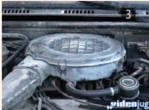
Fig : Cleaning of air filter housing
